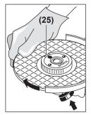
Press the spindle lock button (1) to lock the grinding spindle. To tighten the quick-clamping nut, turn the grinding disc firmly clockwise.
