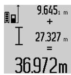
To call up the sum of both measurements, press the result button **6**. The calculation is indicated in the measured-value lines **a**, and the sum in the result line **c**.
