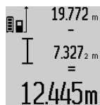
To subtract measuring values, press minus button **5**. For confirmation, “**-**” is indicated on the display. The further procedure is analog to “Adding Measured Values”.
