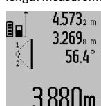
Upon completion of the measurement, the result for the sought distance "X" is displayed in the result line **c**. The measuring values for the distances "1", "2" and the angle "a" are displayed in the measured-value lines **a**.
