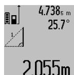
Upon completion of the measurement, the result for the sought distance "X" is displayed in the result line **c**. The measuring values for the distance "1" and the angle "a" are displayed in the measured-value lines **a**.
