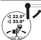
To adjust the standard bevel angle (22.5° and 33.9°), the locking lever must be released upwards.
