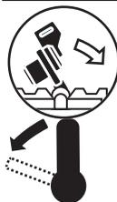
In order to adjust the right-hand bevel angle range, you must first tilt the tool arm slightly to the left and then push the adjusting lever to the left.
