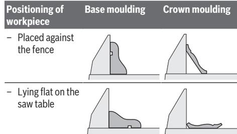
Furthermore, you can cut with or without the slide movement depending on the width of the moulding.
